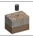
In the floor, insert and glue with silicone the formwork
