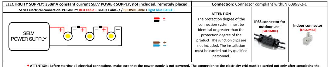
wiring of all the components. If this simply rule is not respected, the lighting source will be irremediably damaged. The installation must be carried out by qualified personnel.
