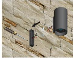
Carry out the electrical connection of the Led lighting body paying attention to the cables polarity and fix it to the support by the provided screws
