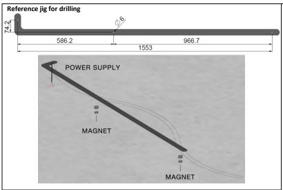
Define the lamp position. Arrange the jig to the wall/ceiling to define position of the electricity supply hole and of the two magnets.
