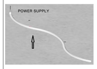
Connect the power cables to the lamp, align and place the lamp supports in the magnets positions.
