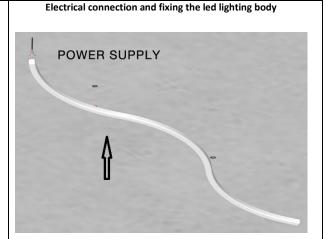
Connect the power cables to the lamp, align and place the lamp supports in the magnets positions.
