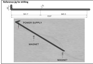
Define the lamp position. Arrange the jig to the wall/ceiling to define position of the electricity supply hole and of the two magnets.
