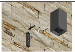
Carry out the electrical connection of the Led lighting body and fix it to the support
