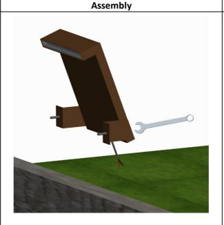
Do the electrical connection and fix with plugs for screws maximum diameter 8mm.
