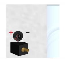
Carry out the electrical connection paying attention to the polarity of the power cables
