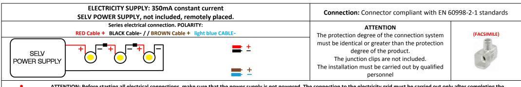
ATTENTION: Before starting all electrical connections, make sure that the power supply is not powered. The connection to the electricity grid must be carried out only after completing the wiring of all the components. If this simply rule is not respected, the lighting source will be irremediably damaged. The installation must be carried out by qualified personnel.
