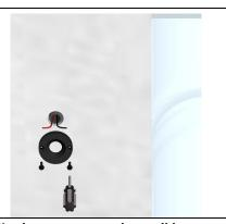
Fix the support to the wall by two countersunk screws maximum diameter 3,5mm
